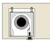
This is similar to the shadow gap (above), although the bottom bar remains visible and does not fully retract through the ceiling opening. However, the headbox is fully hidden from sight. The bottom bar car be powder coated to match the ceiling color. The ceiling material needs to withstand the pressure of stopping the curtain in its resting position. This works with the FA model curtain.
