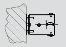
For curtains mounted on the inside of an opening that will not have a niche framed in to hide the side guide.
