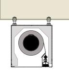
The headbox will be visible. This applies when there is no room for the headbox above the finished ceiling or when it's impossible to build a soffit. Also, the headbox can be installed directly above an opening, reducing the curtain drop when aesthetics is not critical.
