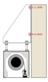
This is the most straightforward method of headbox mounting if there is enough wall space above the headbox assembly. The brackets can mount on concrete, CMU, or wood.
