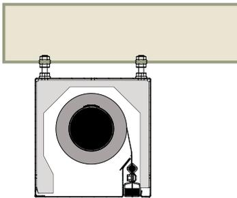
The headbox can be mounted overhead with or without a bracket. The unit can be attached directly to wood framing or concrete, or suspended from steel beams or a metal framing systems such as Unistrut.
