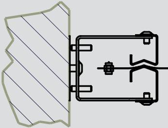
For curtains mounted on the inside of an opening that will not have a niche framed in to hide the side guide.
