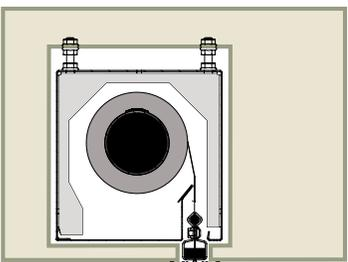
This is similar to the shadow gap (above), although the bottom bar remains visible and does not fully retract through the ceiling opening. However, the headbox is fully hidden from sight. The bottom bar can be powder coated to match the ceiling color. The ceiling material needs to withstand the pressure of stopping the curtain in its resting position. This works with the FA model curtain.
