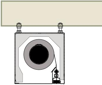
The headbox will be visible. This applies when there is no room for the headbox above the finished ceiling or when it's impossible to build a soffit. Also, the headbox can be installed directly above an opening, reducing the curtain drop when aesthetics is not critical.
