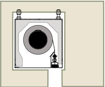
When the headbox is entirely hidden above the ceiling, the bottom bar can retract through an opening in the ceiling and be completely hidden, leaving only a shadow gap. Pay special attention to the bottom bar selected and the size of the opening required for the curtain to clear the opening. Large spans will require a larger aperture to allow the curtain to clear the gap without contact. Most often used with SD curtain.
