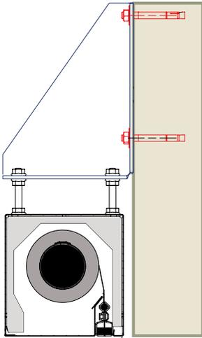
This is the most straightforward method of headbox mounting if there is enough wall space above the headbox assembly. The brackets can mount on concrete, CMU, or wood.
