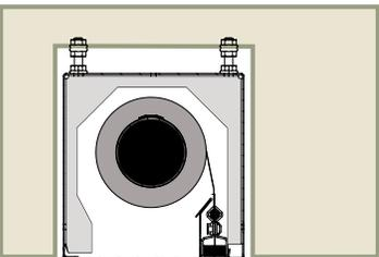
This provides good aesthetics while allowing for simple installation and easy access to the headbox for installation and maintenance. Only the bottom of the headbox is exposed, and the unit can be powder coated to match the surrounding ceilings or walls.
